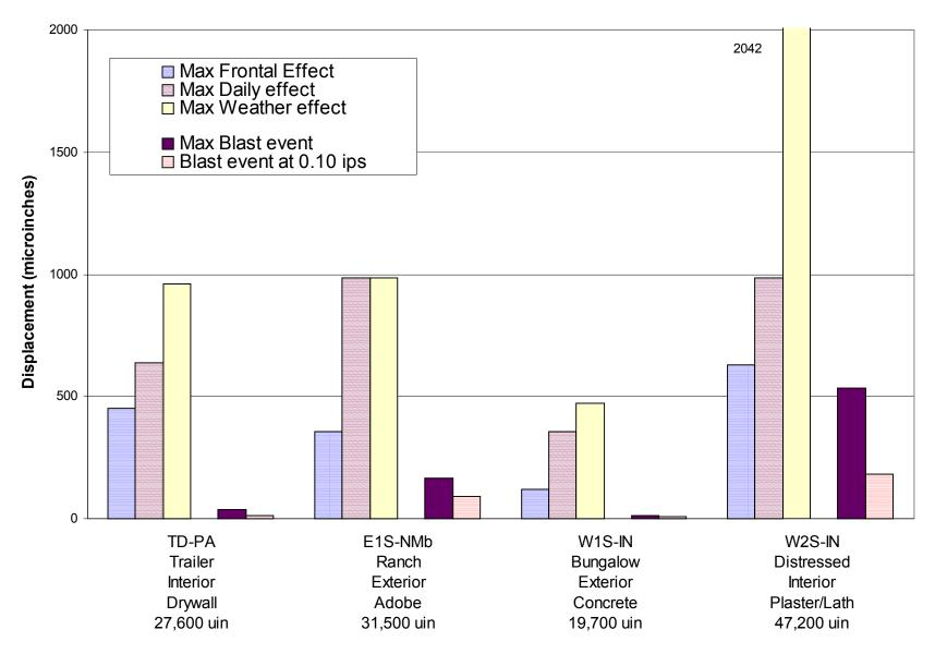
Figure 12 Comparison of measured crack displacements due to static and dynamic events
