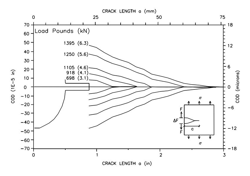
Figure 2 Experimental verification of proportionality of crack width and length
