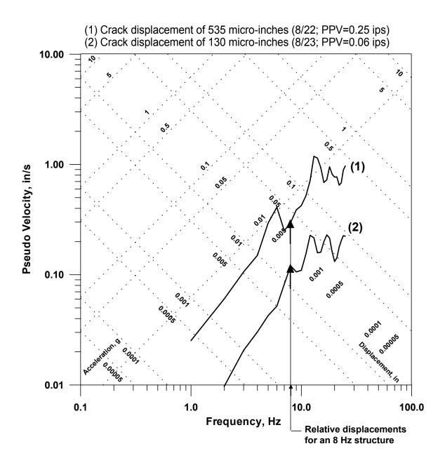
Figure 8 Single degree of freedom response spectra of transverse motions produced by blasts on 22 August 2001 at 17:30 and 23 August 2001 at 13:00, showing estimated relative displacements of an 8 Hz structure
