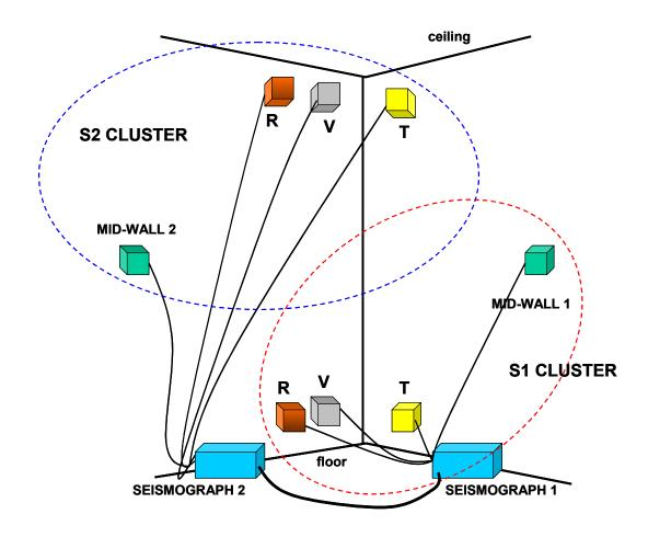
Figure 5 Typical indoor velocity transducer and seismograph set-up (Martell, 2002)
