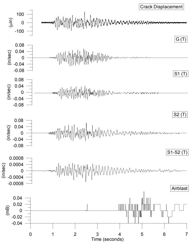
Figure 7 Time histories of crack displacement on 23 August 2001 at 13:00 compared to transverse ground, S1, and S2 structure motions, calculated displacement of the structure (S1-S2)T, and air blast response
