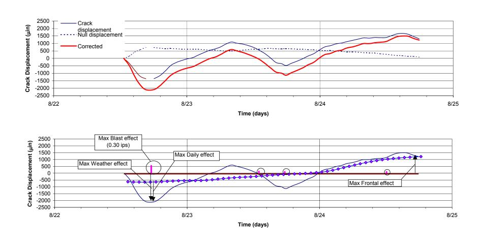
Figure 10 Typical crack response due to long-term phenomena and maximum zero to peak dynamic blast events
