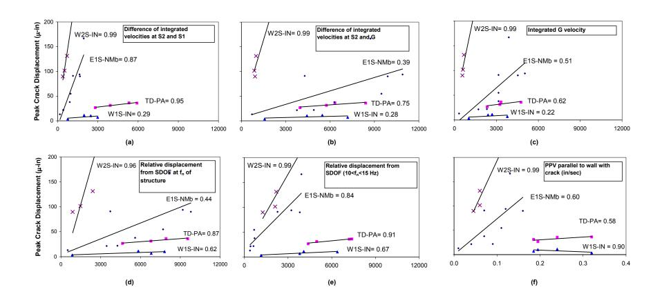
Figure 13 Comparison of R<sup>2</sup> correlations between measured crack displacements and estimated displacements and peak parallel ground motions
