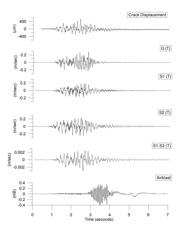
Figure 6 Time histories of crack displacement on 22 August 2001 at 17:30 compared to transverse ground, S1, and S2 structure motions, calculated displacement of the structure (S1-S2 )T, and air blast response
