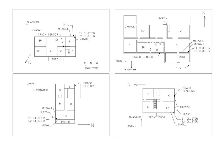
Figure 4 Plan views of four structures monitored for crack response to long-term and transient effects (clockwise from top left: TD-PA, E1S-NMB, W2S-IN, and W1S-IN)
